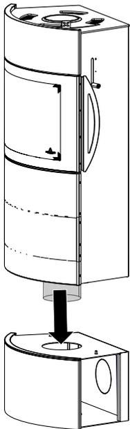
Fig. 26: Placing the stove on to the base
