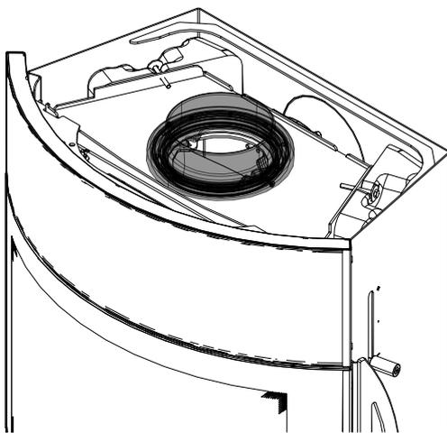
Fig. 39: Installing the rotary flue pipe bracket
