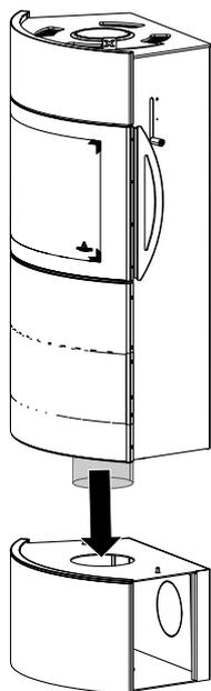
Fig. 21: Placing the stove on to the base
