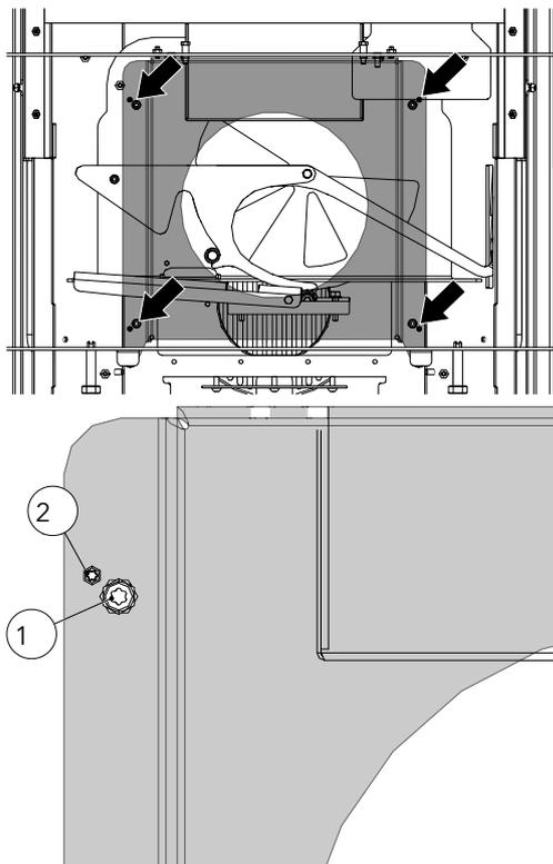
Fig. 52: Adjusting the trim at the bottom
