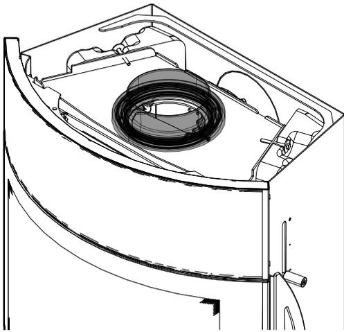
Fig. 45: Installing the rotary flue pipe bracket
