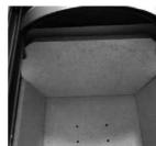
Baffle in position resting on supports.
