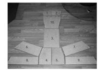
Left inner top baffle bricks 1 positioned on secondary air pipe & side supports.
